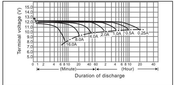
**Duration of discharge vs. Discharge current <sup>(note)</sup>**
