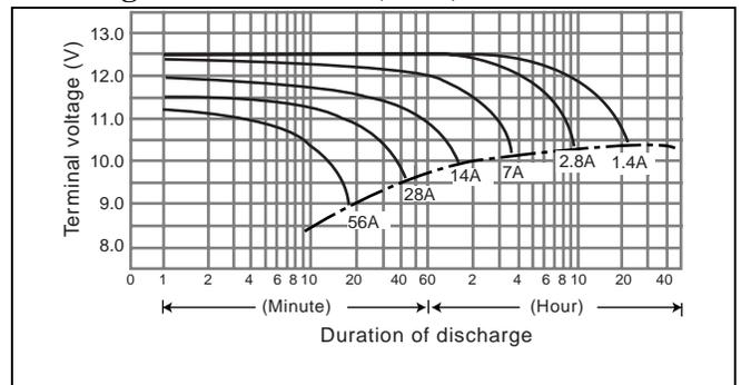
**Duration of discharge vs. Discharge current <sup>(note)</sup>**
