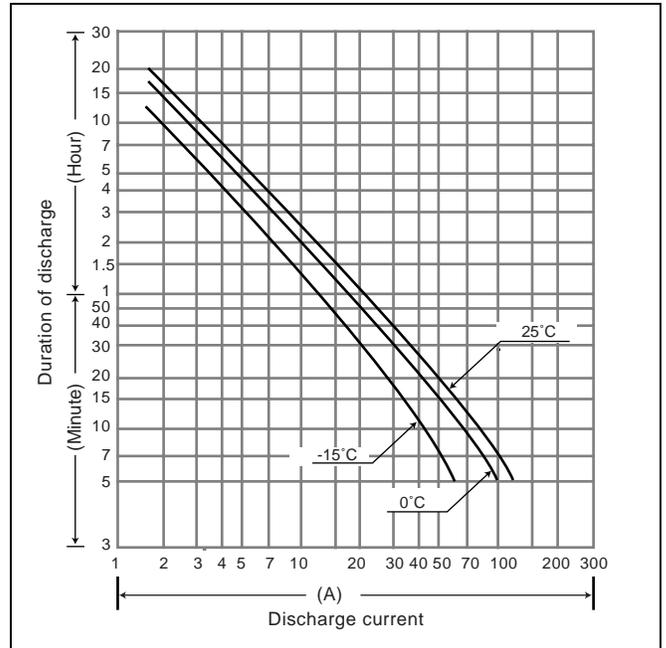
(Note) The above characteristics data are average values obtained within three charge/discharge Cycles not the minimum values.
