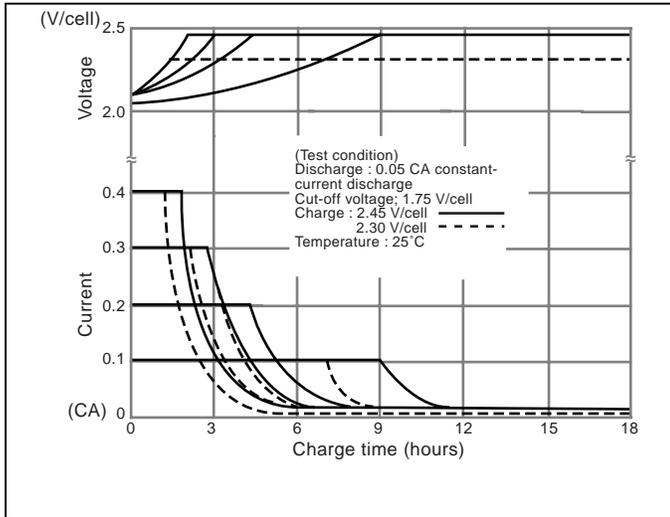
In order to fully utilize the characteristics of SLA batteries, constant-voltage charging is recommended. For details of charging see page 20.
