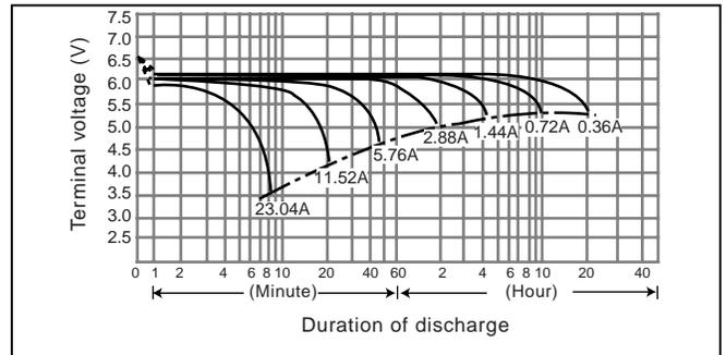
**Duration of discharge vs. Discharge current <sup>(note)</sup>**
