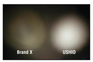
**Brand X** – Uneven beam pattern, low color temperature, green color and low output
