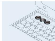
The VARTA HyRate "Bridging" batteries maintain the PC partially operational at reduced power levels during exchange of the main battery or during some periods of work interruption.
