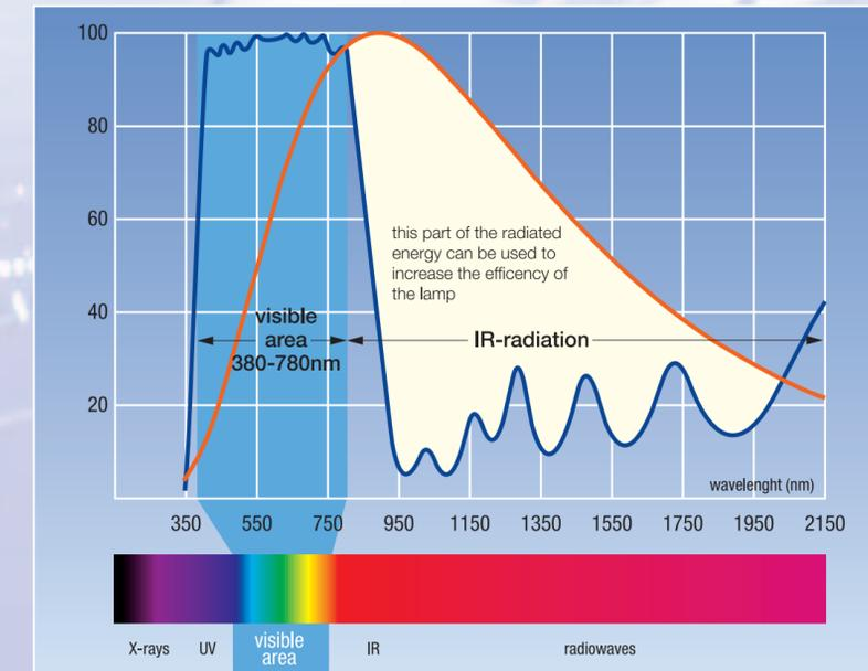
Figure 2: IRC-Airfield lamps, sphere of activity
