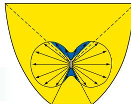
Axial, low stray light portion: approximately 30% higher luminous efficiency can be attained by axial arrangement
