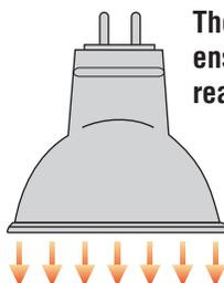
The aluminum coating of the reflector ensures lower heat radiation to the rear of the lamp
