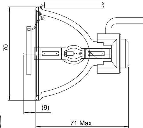
Lamp aligned for max throughput thru 6mm aperture at 52mm dist from reflector rim.
